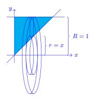
The inner radius of the washer is r = x. (This is the distance from the x-axis to the line y = x.) The outer radius of the washer is R = 1. (This is the distance from the x-axis to the line y = 1.) The thickness of the washer is dx. Thus, the volume element is the volume of the washer:
